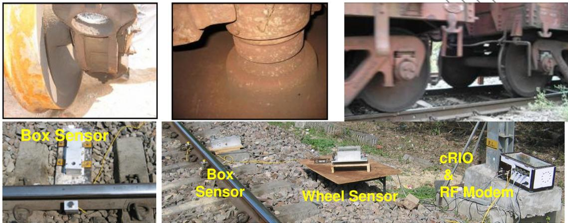
After processing in the cRIO chassis the signals are then sent through the modem to the mother computer in Control Office or TXR's Office. cRIO comes equipped with both Ethernet and RS232C (and now also USB) ports; any of them can be used for the interface.
