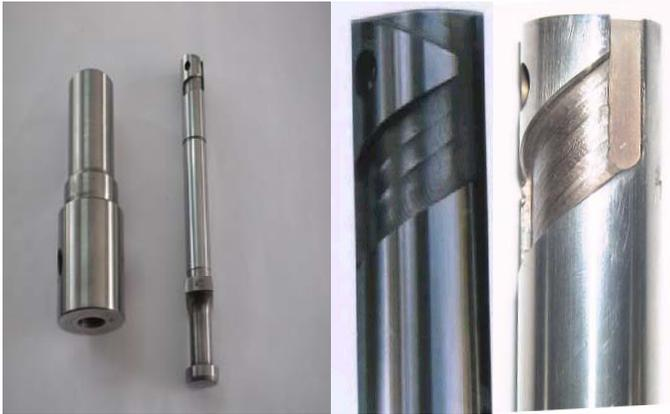
Figure 7: Barrel and plunger of Double Helix Fuel Injection pump, double helix and single helix plungers
